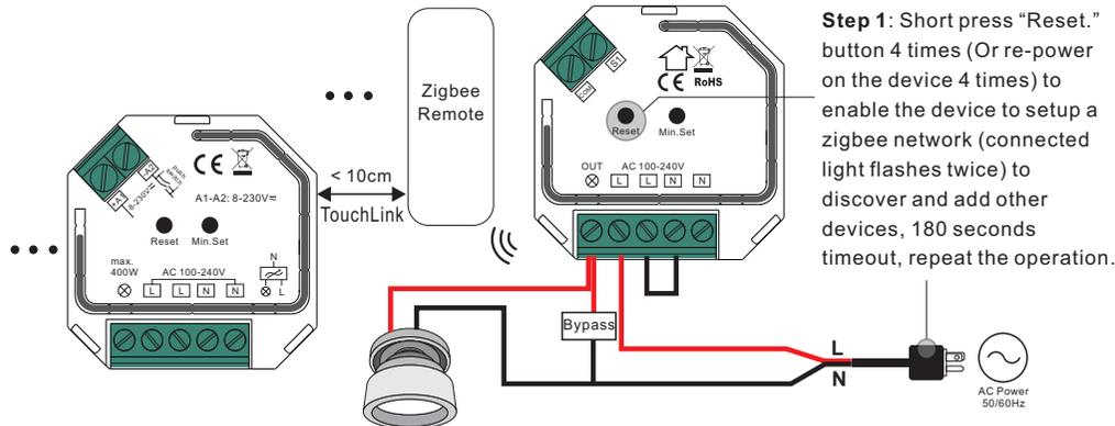
**Step 1:** Short press "Reset." button 4 times (Or re-power on the device 4 times) to enable the device to setup a zigbee network (connected light flashes twice) to discover and add other devices, 180 seconds timeout, repeat the operation.
