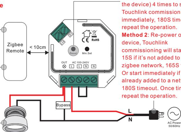
**Step 1: Method 1:** Short press "Reset" button (or re-power on the device) 4 times to start Touchlink commissioning immediately, 180S timeout, repeat the operation.
