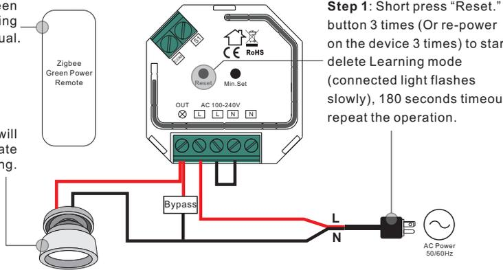
**Step 1:** Short press "Reset." button 3 times (Or re-power on the device 3 times) to start delete Learning mode (connected light flashes slowly), 180 seconds timeout, repeat the operation.
