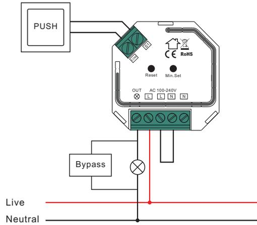
**NOTE:** Switch connected to the S1 terminal activates the basic functionality of the dimmer (turning the light on/off, dimming).
