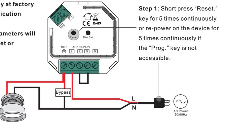
**Step 1:** Short press "Reset." key for 5 times continuously or re-power on the device for 5 times continuously if the "Prog." key is not accessible.
