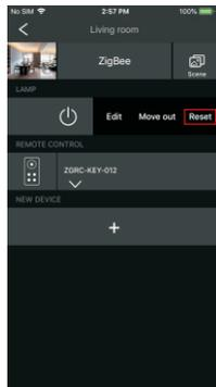
From your ZigBee controller or hub interface, choose to delete or reset the lighting device as instructed. The connected light blinks 3 times to indicate successful reset.
