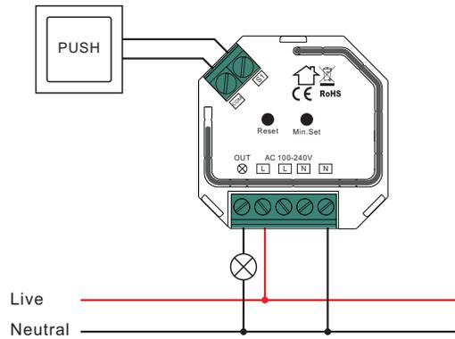
**NOTE:** Switch connected to the S1 terminal activates the basic functionality of the dimmer (turning the light on/off, dimming).
