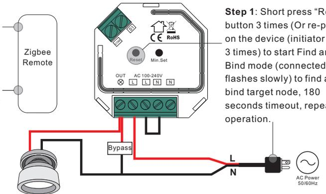
**Step 1:** Short press "Reset." button 3 times (Or re-power on the device (initiator node) 3 times) to start Find and Bind mode (connected light flashes slowly) to find and bind target node, 180 seconds timeout, repeat the operation.
