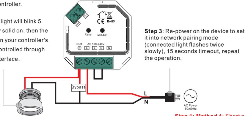
**Step 3:** Re-power on the device to set it into network pairing mode (connected light flashes twice slowly), 15 seconds timeout, repeat the operation.
