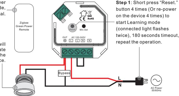
**Step 1:** Short press "Reset." button 4 times (Or re-power on the device 4 times) to start Learning mode (connected light flashes twice), 180 seconds timeout, repeat the operation.
