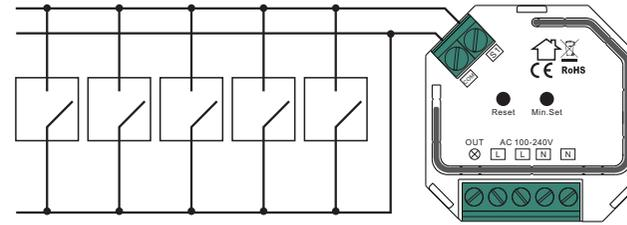
This phase dimmer adopts leading edge dimming (forward phase control) or trailing edge dimming (reverse phase control), two versions are available for choosing, factory default version is trailing edge. Please make sure the connected loads support the control type you choose. Please refer to the user manual of the load or consult the supplier of the load.
